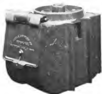
Fig. 4486. Gould Journal Box with Inset Lid and Dust Guard, Type M-O, for Pedestal Trucks.
